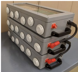
Figure 8. RDT-Equipped, 300-cell Full Battery Demonstrator.
