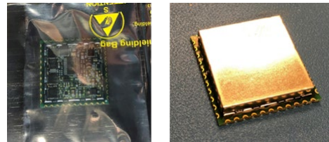
Figure 10. (Left) RDT Core unit circuit board (1.2' x1.2"). (Right) With protective cover fitted.
