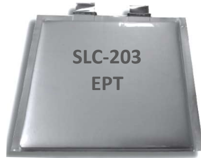
Figure 5. Picture of 13Ah SLC203 cell
