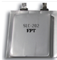
Figure 1. Picture of SLC-202 cell (2.3Ah)
