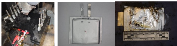
Figure 7. Nail penetration results of SAFT BB-2590 LMFP cell with semi-solid state gel polymer electrolyte (left) compared to an NMC based cell (right)
