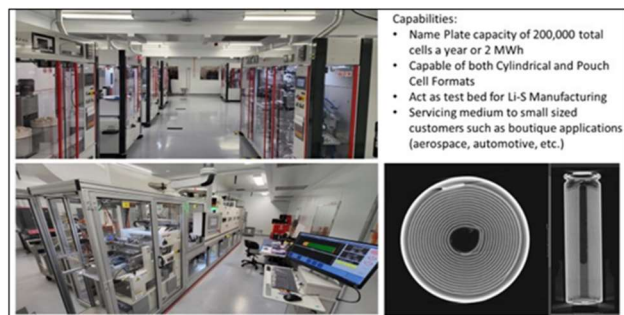
Fig. 9. Pilot lines for assembling MLP (10Ah) and 18650/2170/26650 cylindrical Li-S cells
