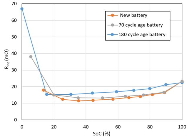
**Figure 4.**  $R_{\text{int}}$  vs. %SoC @ 10-hour step discharge rate for new battery, 70 cycle age battery, and 180-cycle-age battery.
