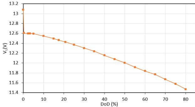
**Figure 2.**  $V_L$  vs %DoD @ 10-hr rate up to EODV=10.8V;  $V_L$  (min) = 11.375V; Ah max = 192.953 at EODV=10.8V
