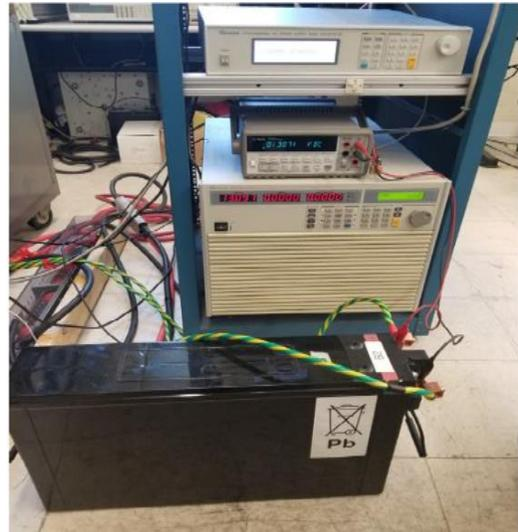
**Figure 1.** Experimental setup for battery auto cycling and battery characterization.
