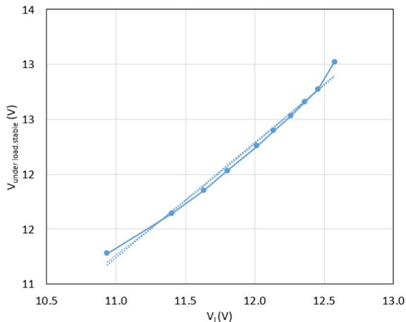
**Figure 3.**  $V_{\text{under load.stable}}$  vs  $V_L$  for a NEW battery @ 10-hour step discharge rate up to EODV=10.8V;  $V_L$  = battery voltage during discharge.
