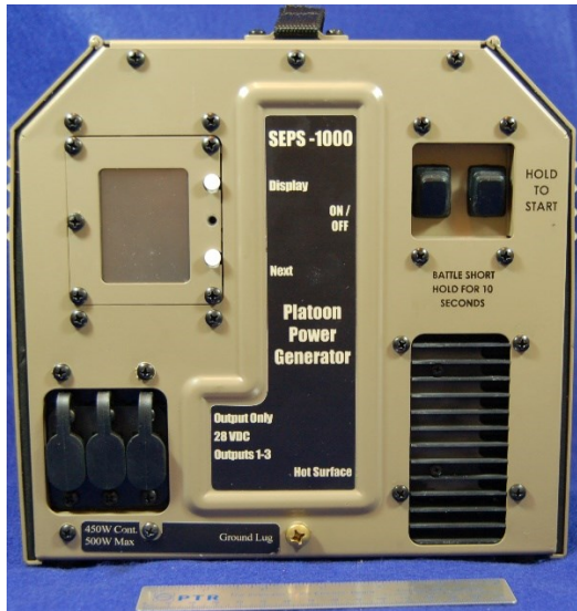
Figure 1. Platoon Power Generator. Scale in foreground is 6 inches wide. 28VDC (450W / 500W Peak).
