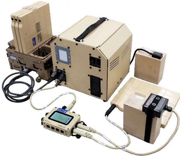
Figure 4. Complete PPG System including Generator, UBC, and SPM.
