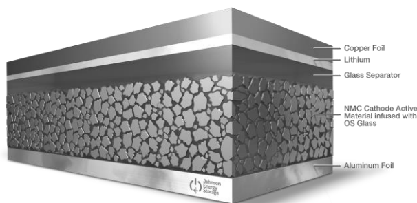
Figure 1: Illustration of the cell configuration utilized by Johnson Energy Storage.
