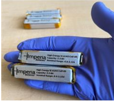
Figure 2. nUAS Cells achieving >300 Wh/kg. Cell weight <31 grams with equivalent size (LxWxH) to 18650 battery.
