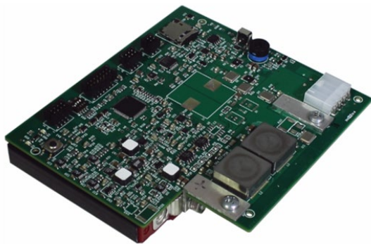
Figure 5: ESL Hybrid Power Management Board and Lithium-Ion Supercapacitor
