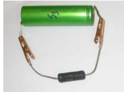
Fig. 4 Photograph of 18650 test cell with a 20-ohm resistor under 0V storage test
