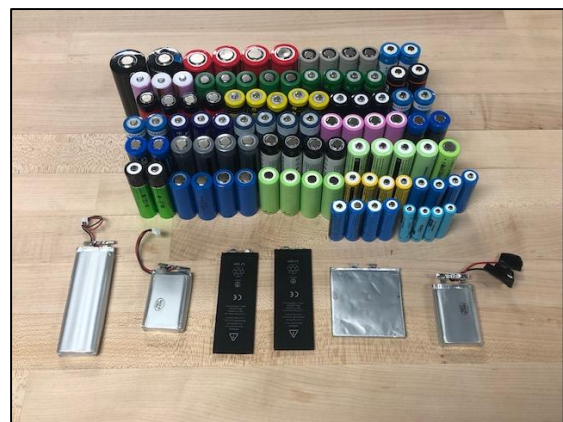
Figure 3. Collection of some of the pouch and cylindrical cells evaluated in this study
