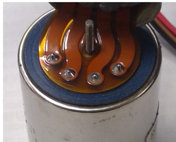
Figure 2: Soldered flex harness on a Thermal Battery.
