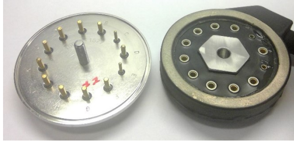
Figure 3: Custom solution with threaded stud surrounded by contacts.
