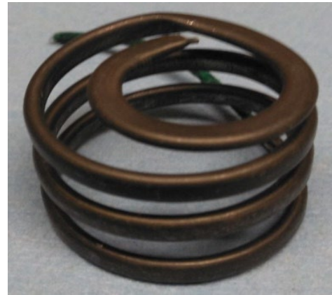
Figure 2: A coiled and consolidated heating fuse section with integral helical cap section.
