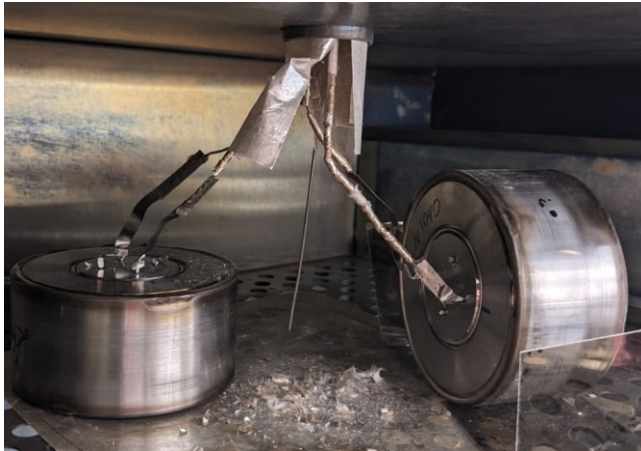
Figure 2. Photograph Of the Units, One Set on the Baseplate and One on the Side, Under Test in the Oven.
