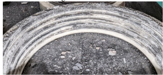
Figure 5. DPA Photo of the Sleeve Contamination.
