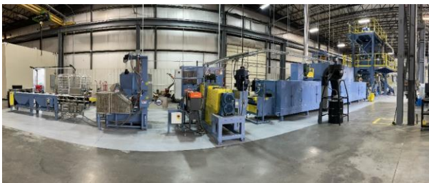
Figure 5: Advancement in the manufacturing process of NiZn cathodes: From manual tape caster to automated coater.
