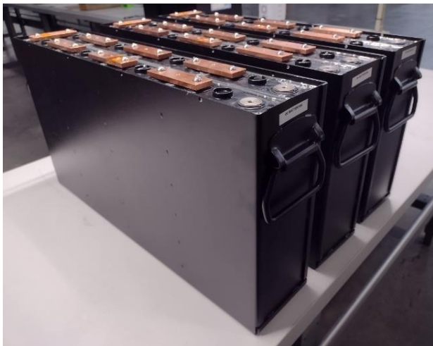
Figure 3: Three 12V NiZn prototype batteries made for high-rate standby applications. Each battery contains 8 NiZn cells.
