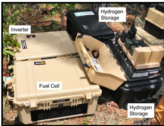
Figure 3. Hydrogen Small Unit Power Prototype
