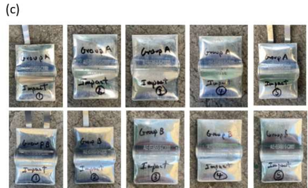
Figure 4. (a) Group A impact test with temperature and voltage recorded (b) group B impact test with temperature and voltage recorded (c) Cell images after impact test
