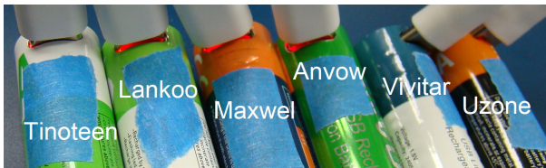
Figure 9. All USB-C batteries had a red LED that blinks through the USB-C connector when charging. The LED stays on when fully charged.
