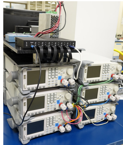
Figure 2. Part of the test stand used for this study. Includes the e-loads, USB hub, and thermocouple reader.
