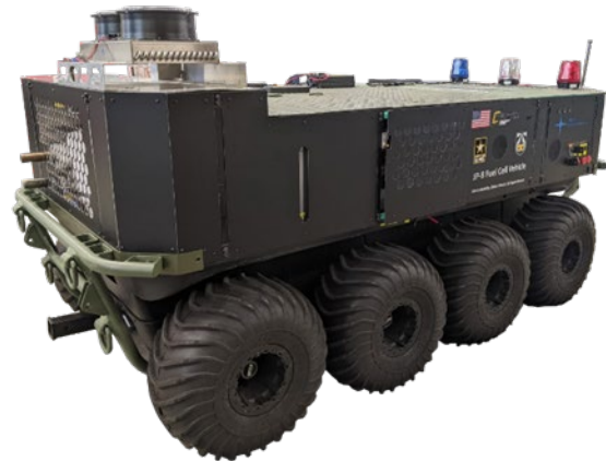
Figure 1. F-24/JP-8 fueled, electric SMET prototype developed at PCI with US ARMY DEVCOM GVSC support. It is self-charging and provides 10-kWe export power.
