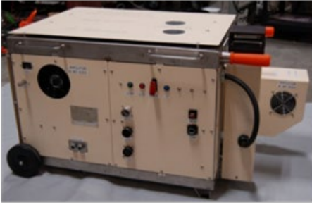
Figure 2. 1.2 kW JP-8/Diesel fueled SOFC generator prototype developed with USTRANSCOM support.
