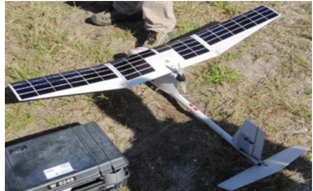
Fig 2. Air Force Research Laboratory partnership with UES, Inc. and Microlink Devices, Inc., has integrated new lightweight, flexible, high-efficiency solar panels onto a small, unmanned aircraft system (UAS) platform [4-5].
