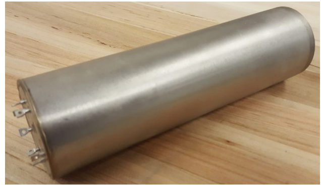
Figure 6. Thermal Battery B Configuration
