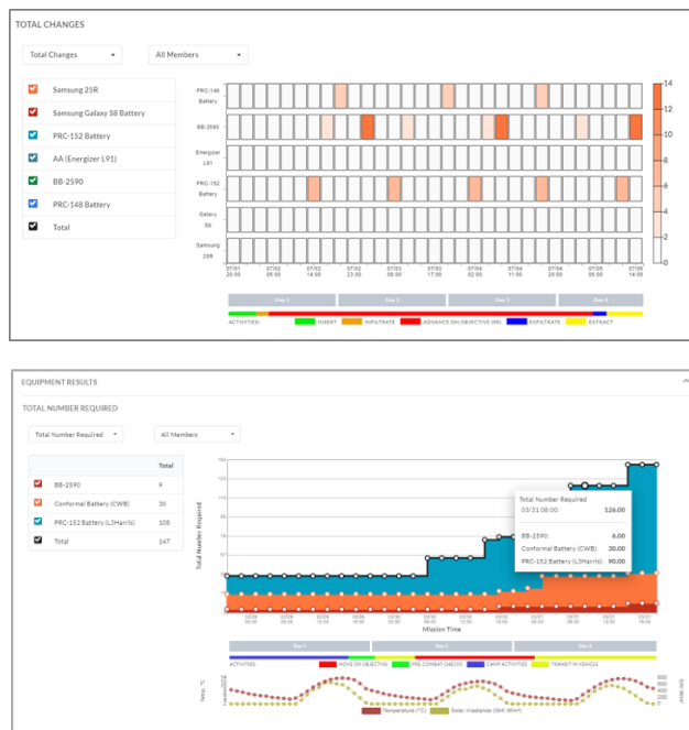
Figure 4. UI examples. A heat map showing when and how many batteries are replaced (top) and a plot of the number of batteries required as a function of mission time (bottom).
