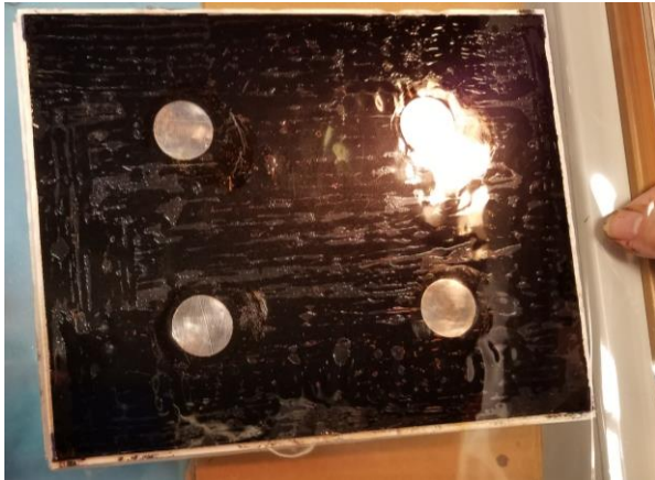
Figure 5. Single full scale 6TAGM pouch cell electrode, rear face with.
