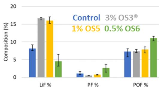
**Figure 6: Fluorine components after formation (Si anode).**
