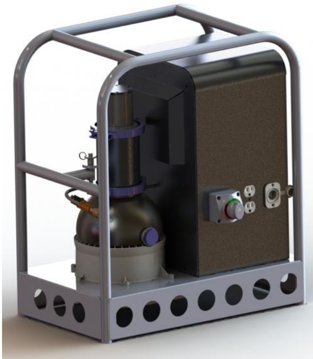
Figure 2. Design rendering of TDA's hydrogen-fueled portable power generator. The gas production unit with a spherical reactor is located at the front of the generator, and the fuel cell and power outputs are housed in the casing. An aluminum frame protects the generator.
